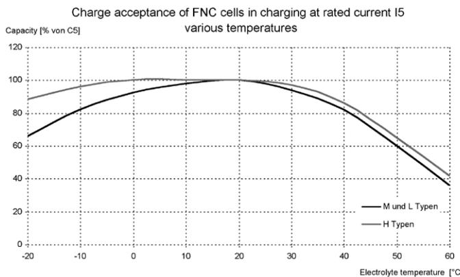
If batteries with cells of type L are correctly charged at an electrolyte temperature of -20°C, then only 66% of the rated C<sub>n</sub> can be fed into the battery. These cells also display the same behaviour at higher temperatures: at 45°C the battery can be charged to only 70% of rated capacity C<sub>n</sub>.
