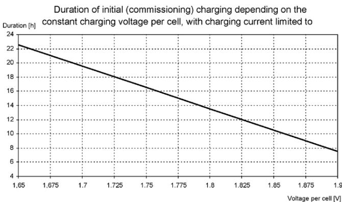
If now the current is also limited, then charging time must be further extended. For a battery charged with a limitation of cell voltage to 1.8 V per cell and a current of  $I_5$ , then 13.5 hours will be required to obtain a good result. If the current is halved, then the charging time must be doubled.
