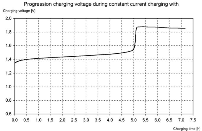
In principle, HOPPECKE recommend commissioning at constant current  $I_5$  for all NiCd cells, but commissioning with constant voltage is also possible. The state of full charge of an alkaline battery is clearly recognisable from a rise in voltage. During initial charging with constant current, cell voltages up to 1.9 V may occur. The charging method used in commissioning must allow for this and, where necessary, the battery should be split for this purpose.
